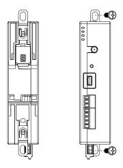
• Installing and dismantling aluminum DIN rail: Attach the back trench of the device to the mounting rail in arrow ① direction and push the device against the rail in arrow ② direction. To dismantle, first push down the device in arrow ① direction and follow arrow ③ direction to release the device.
